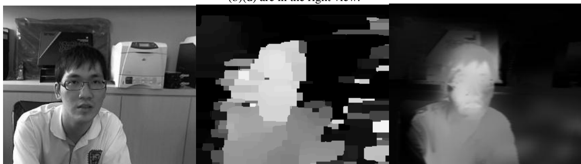
Figure 3. Post processing for depth map. (a) input capture (b) poor quality depth map without post processing (c) depth map with post processing
