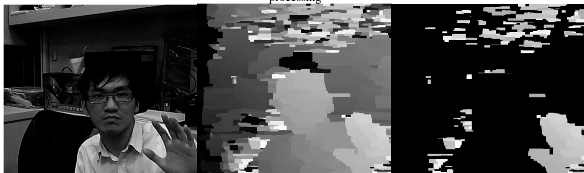
Figure 4. Filter out the background only by depth of user's face. (a) input capture (b) poor quality depth map (c) filter out the background only by depth of user's face
